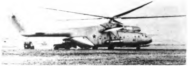
Figure 6-58. Mi-6 HOOK. This heavy-duty helicopter provides lift for 65 troops and about 16.5 tons of cargo. The short stub-wings are a distinctive feature.
